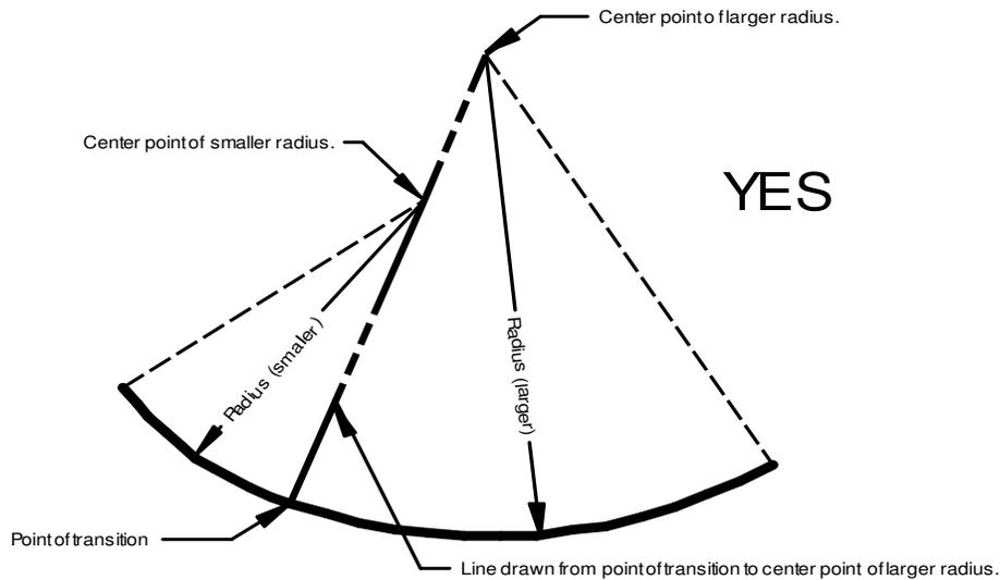
When two concave or convex radius edges of different radii come together the center point of the smaller radius must fall on a line drawn from the point of transition to the center of the radius of the larger radius.
