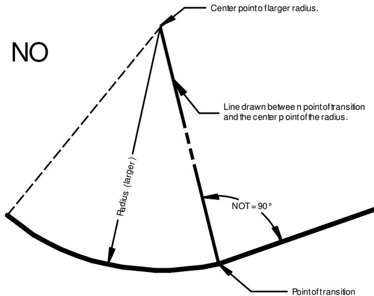
The straightedge NOT at a right angle to a line drawn from the point of transition to the center point of the radius.
