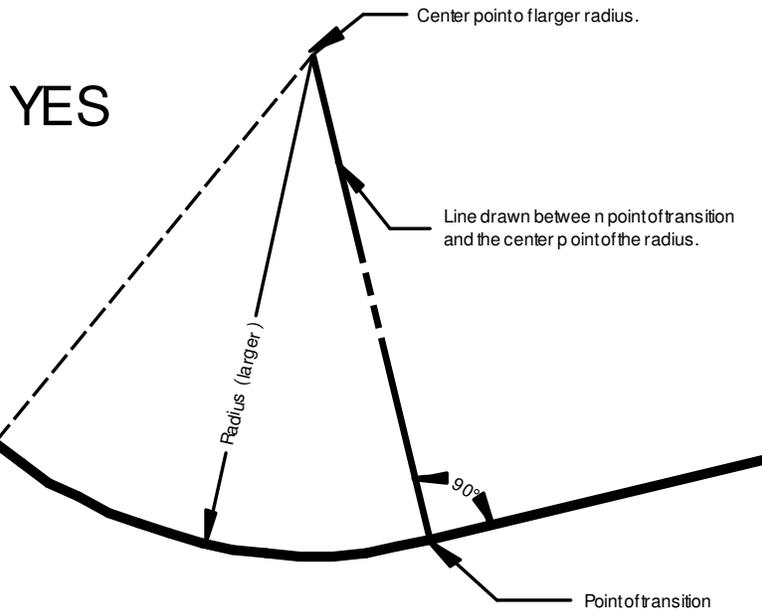
When a concave or convex radius edge come together with a straightedge the straightedge must be at a right angle to a line drawn from the point of transition to the center point of the radius.
