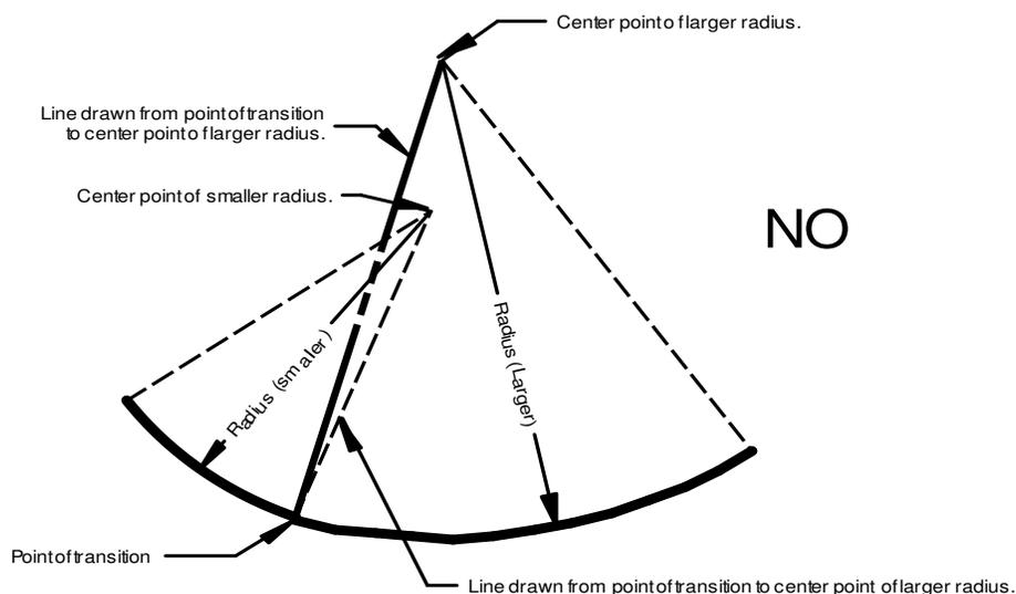
The center point of the smaller radius does NOT fall on a line drawn from the point of transition to the center of the radius of the larger radius.
