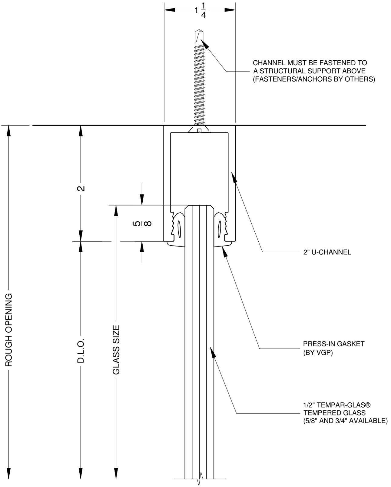
CHANNEL MUST BE FASTENED TO A STRUCTURAL SUPPORT ABOVE (FASTENERS/ANCHORS BY OTHERS)
